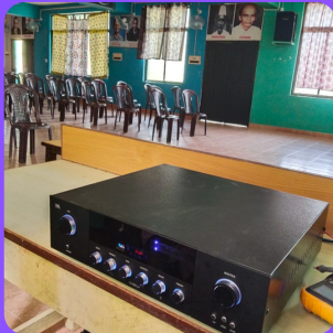
Self designed 600 W MOSFET Hi-fi power amplifiers for auditorium
